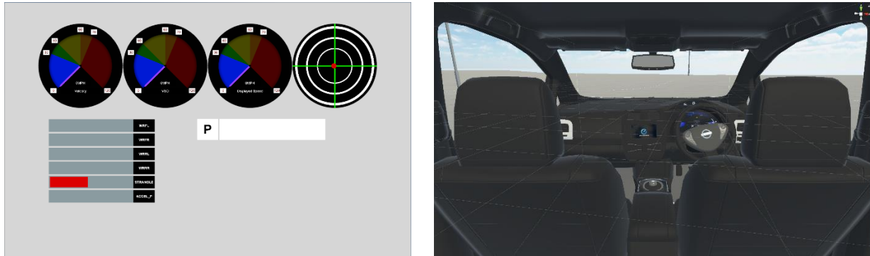
Figure 12: Vehicle stationary (speed and acceleration are zero), with wheel turned slightly left. Interior view of virtual vehicle shown to illustrate how the viewing position can be adjusted as required
